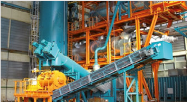
Photo 45: Indirectly Heated Discontinuous Vacuum Mixer for Mercury Recovery, Including Solidification Mixer (courtesy: econ industries GmbH)
