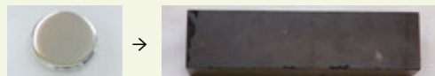
Photo 34: Monolithic Block after the Treatment of Metallic Mercury from the Chlor-alkali Sector
