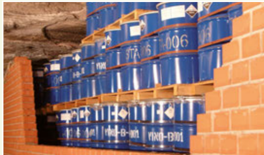
Photo 40: Storage arrangement of drums in the salt mine (courtesy: K+S Entsorgung GmbH)
