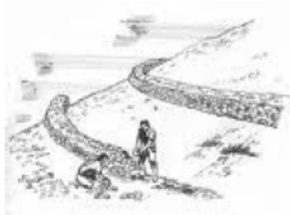
Erosion Control Bunds
