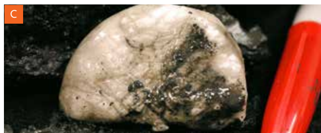
In fine-grained sediment (dark material), gas hydrate (white) can form as large chunks or nodules like the pictured specimen from offshore India.
