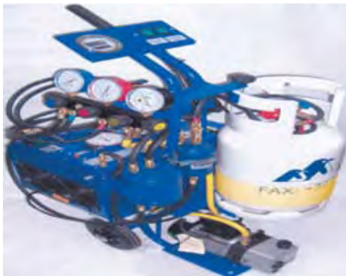
Fig (4-3): Recovery & Recycling equipment for vehicles air conditioning
