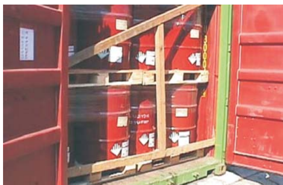
Loading of hazardous waste drums into containers, ready for transport
