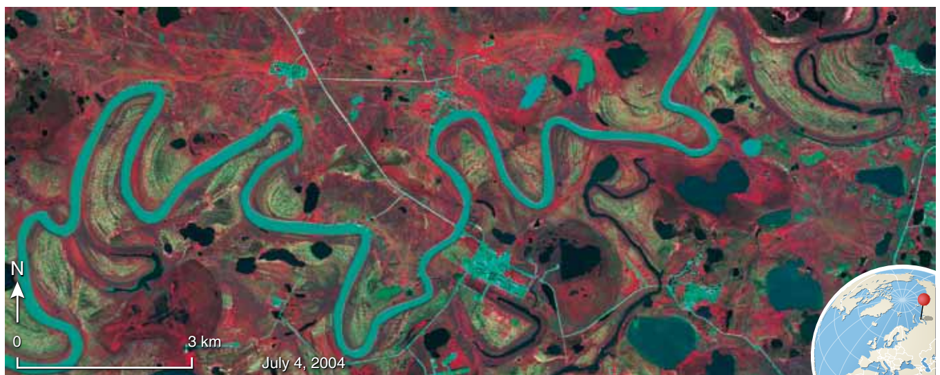
Figure 18.2: A false color Quickbird-2 satellite image of a portion of the Bovanenkovo Gas Field on the Yamal Peninsula in West Siberia. Image acquired 4 July 2004. The construction phase began in the late 1980s. From that period onward there remain visible signs of extensive off-road vehicle traffic across the terrain. Many of those tracks have naturally revegetated and now appear as bright red, indicating dense grass- and sedge-dominated vegetation. The road network was built in the mid-1990s, which has reduced off-road traffic significantly. However, infrastructure blocks segments of migration routes for Nenets and their reindeer herds, and pasture quality can be negatively affected by road dust, petrochemicals, trash left on the tundra, and even feral dogs abandoned by workers [25].
