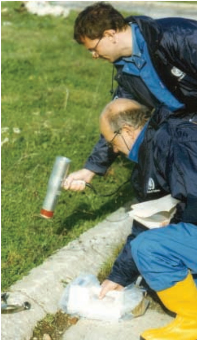
Checking a “contamination point” by measurements of gamma radiation with the Saphymo-SRAT S.P.P. 2 NFscintillometer (left) and the beta radiation by the Berthold Contamination Monitor LB 122 (right).
