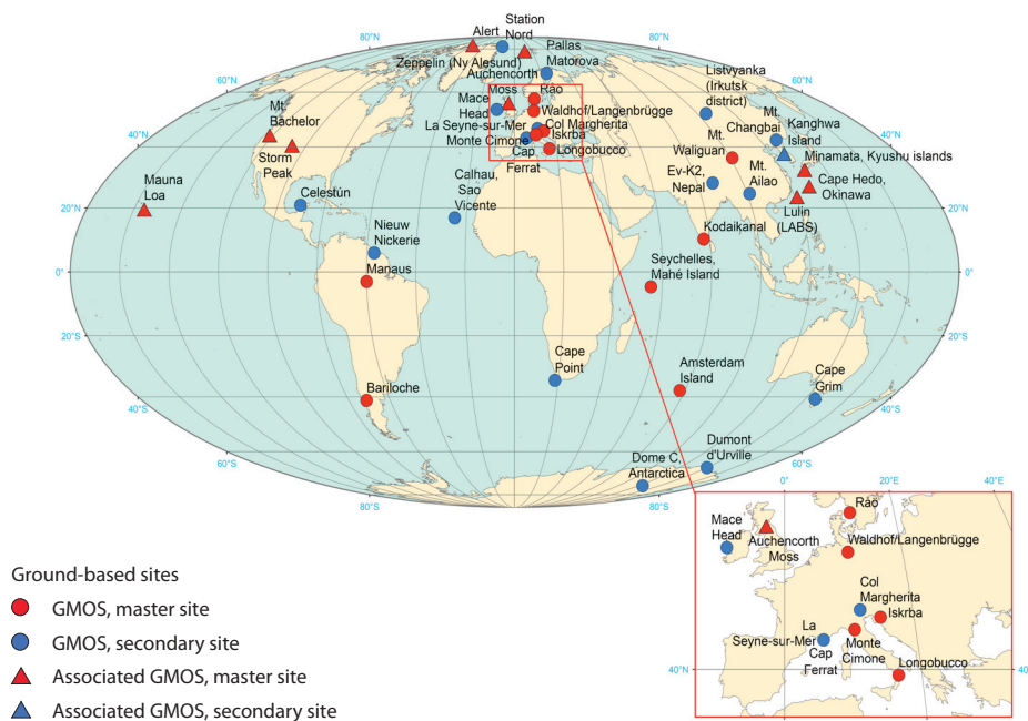
Figure 3.4 Ground-based monitoring sites participating in the GMOS programme ( www.gmos.eu ). GMOS Master sites are those where GEM, GOM, and PBM 2.5 are continuously measured and Hg in rainfall measured where appropriate. Secondary GMOS sites are those where only TGM and Hg in precipitation are continuously measured. Associated GMOS sites are those that are managed by external GMOS partners who have agreed to share their measurement data with the GMOS programme and measurement database.
