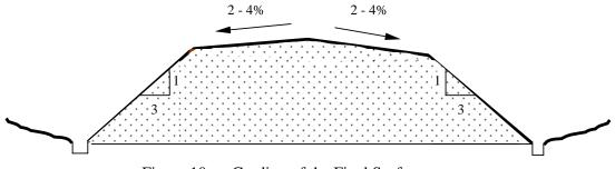
Figure 10. Grading of the Final Surface
