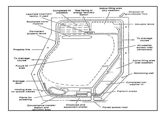
Figure 18. Typical Layout of a Sanitary Landfill
