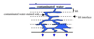
Figure 25. Liquid Flow Through Waste Cell Lifts
