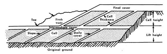
Figure 26. Cross-section of a Completed Landfill
