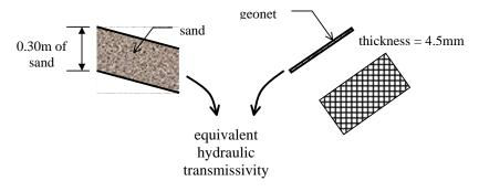
Figure 19. Geonet Compared With a Layer of Sand
