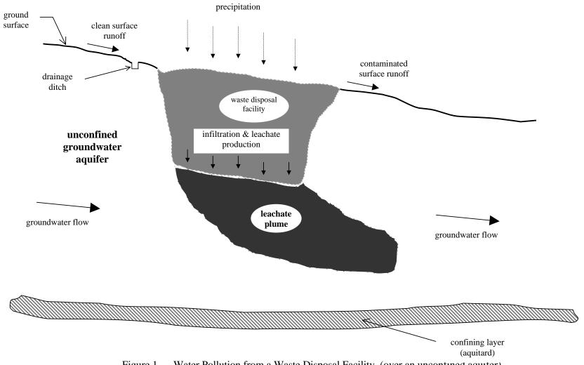
Figure 1. Water Pollution from a Waste Disposal Facility (over an uncontined aquiter)
