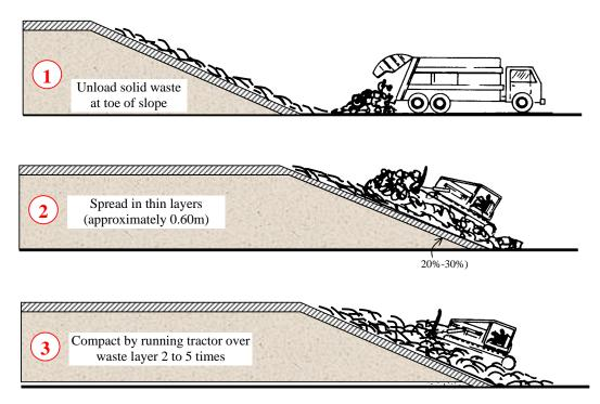
Figure 27. Waste Spreading and Compaction
