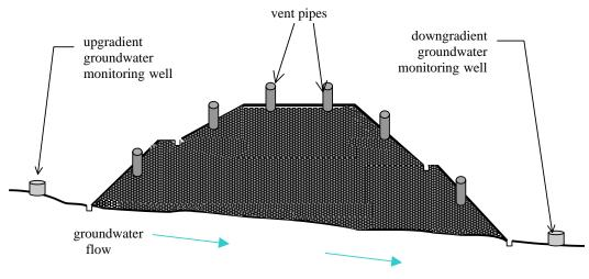
Figure 12. Vent Pipe and Monitoring Well Installation
