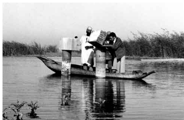
Figure 13 Measuring water levels at Kindjeria (centre of northern pool) in 1975. This gauge is presently not in operation. (Photo: Chouret in USGS 2001)
