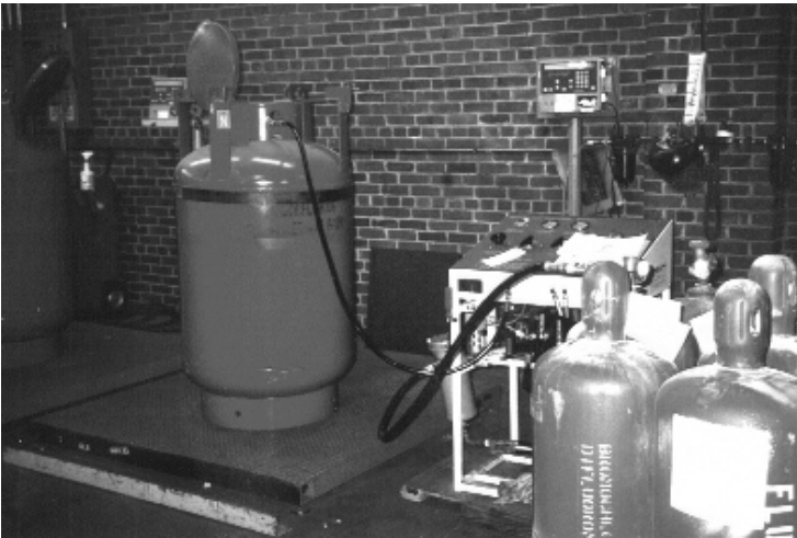
A halon recovery unit in action transferring halon 1211 into a recovery cylinder. Recovery and banking of decommissioned or surplus halon is a key component of a halon management strategy.
