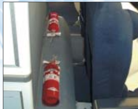
Halotron I extinguishers helping to save the ozone layer and making air travel safer.
