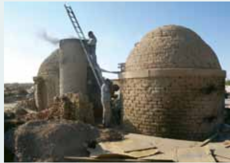
A traditional brick kiln (left) and an improved kiln (right) operating in Mexico
