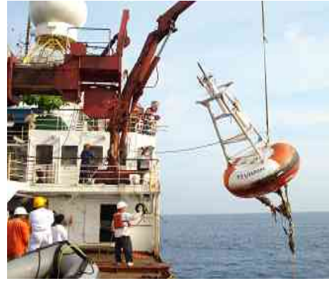
INCOIS buoy deployment during SK-251 in Bay of Bengal
