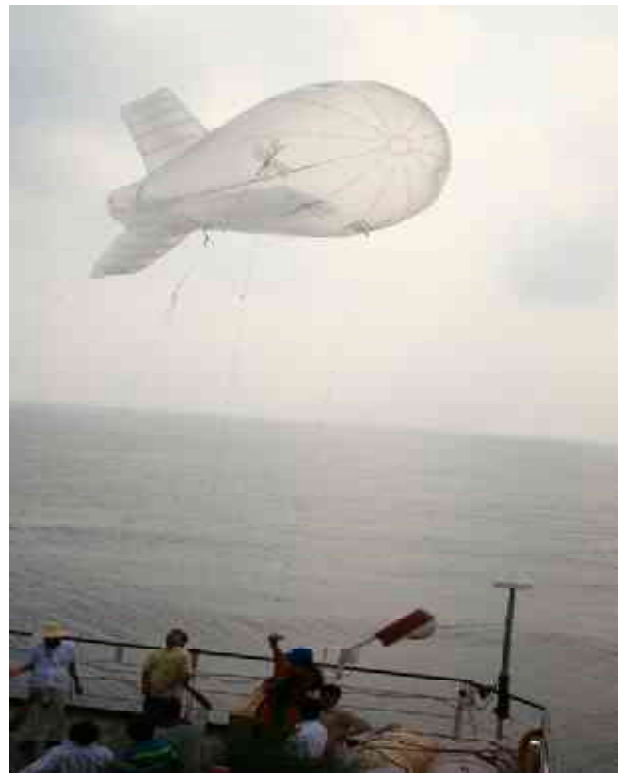
ICARB-Winter Campaign in SK-254: Kytoon tethering for atmospheric studies
