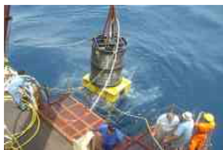
Remotely Operable Submersible Testing from the vessel
