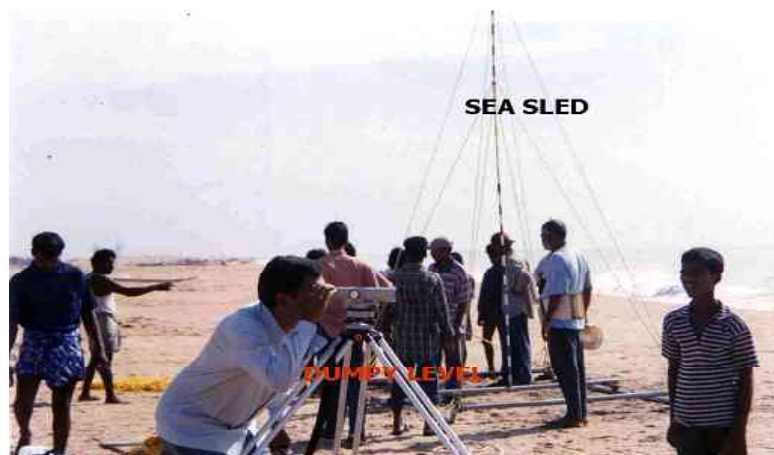
Fig. 2 - Photograph showing the Sea Sled and Dumpy level used for beach profile
