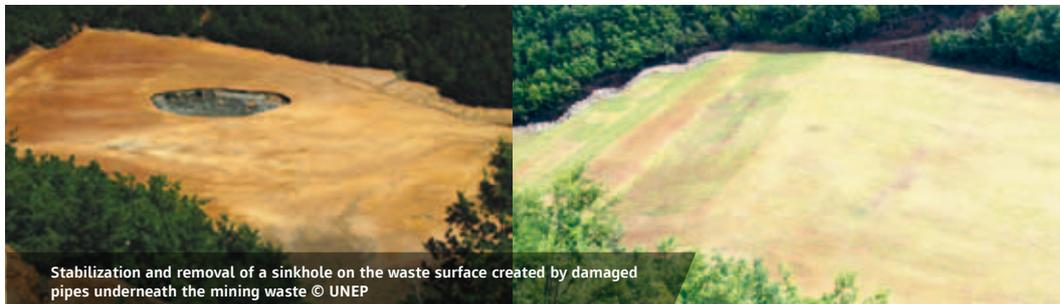
Stabilization and removal of a sinkhole on the waste surface created by damaged pipes underneath the mining waste © UNEP
