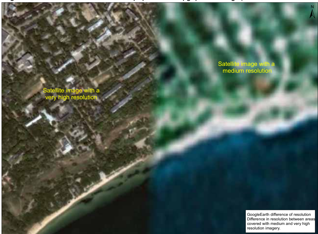
Figure 8. Difference between Quickbird (left) and Landsat (right) satellite imagery for information extraction
