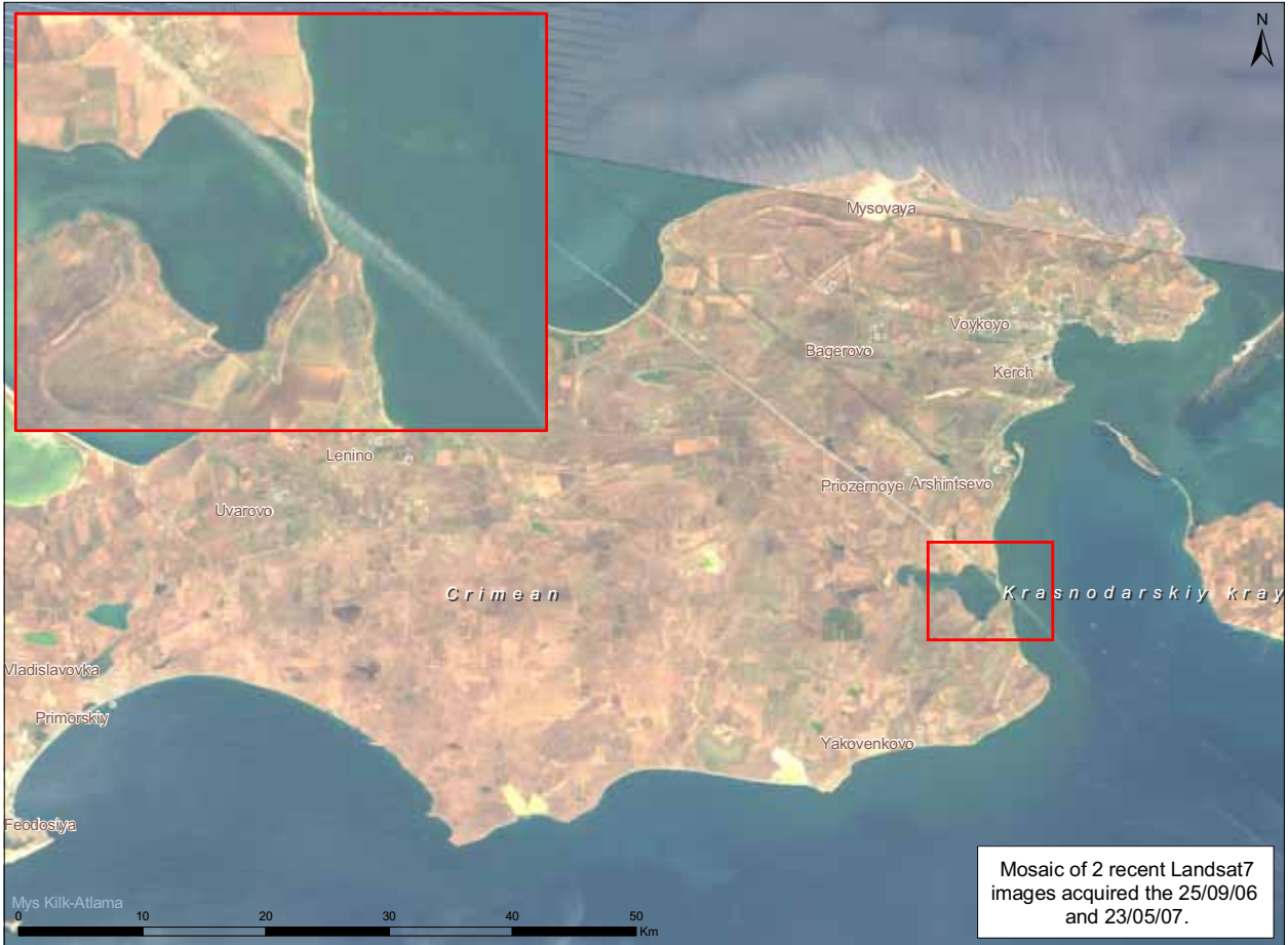
Figure 5. With a resolution of 30 meters/pixel, these Landsat images can be used up to a scale of 1/50,000
