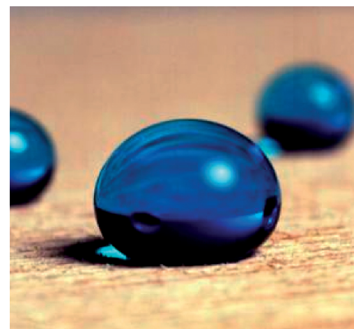
Wood coated with a nanoparticle surface becomes extremely water repellent or 'superhydrophobic'. Surfaces treated in this way become self-cleaning and require little maintenance.
