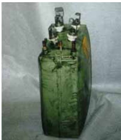
Picture 42: Inflated capacitor
