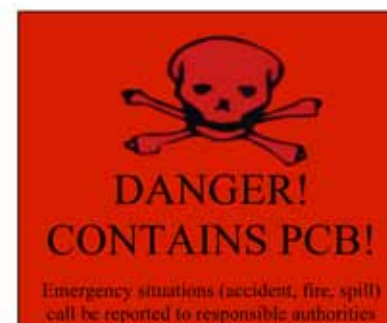
Picture 33: Label for PCB containing equipment
