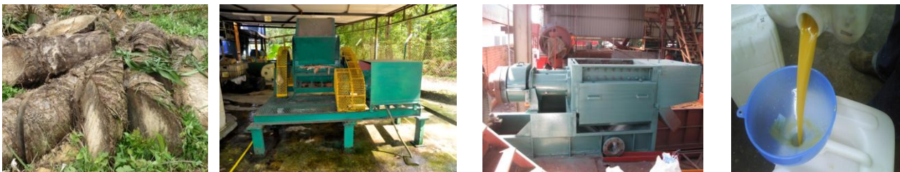
Figure 3.2.3.3 Shredded WPT from fields (left) used for sap extraction on FRIM processing equipment (right)
