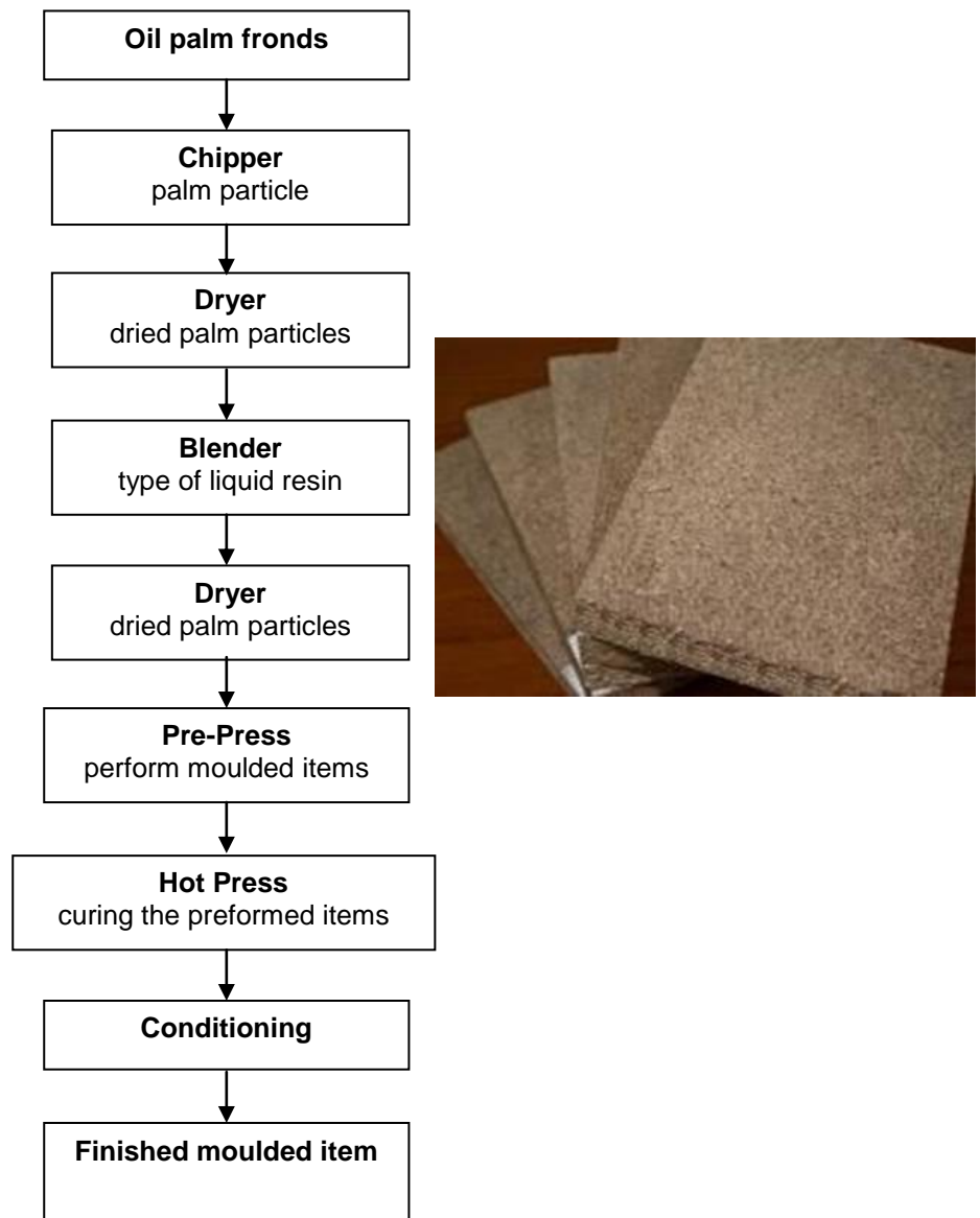
Process flow for no-skin moulded particle board (Asa Naim, 2005)
