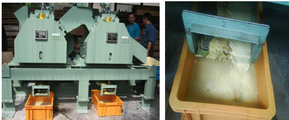
Figure 2.4.2 Oil palm trunk sap squeezing pilot scale equipment (left) and sap produced (right)
