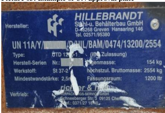
Picture 63: Example of UN approval plate
