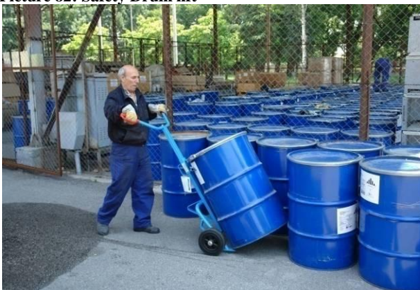
Picture 82: Safety Drum lift
