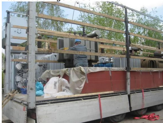
Picture 72: Stowing of transformers
