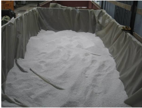
Picture 70: Covering the bottom with absorbent material
