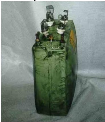
Picture 42: Inflated capacitor
