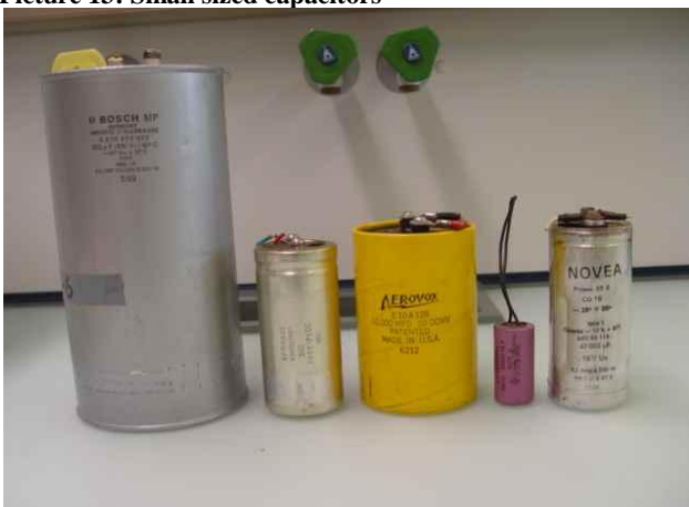
Picture 13: Small sized capacitors
