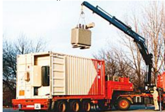
Picture 100: Loading of transformers
