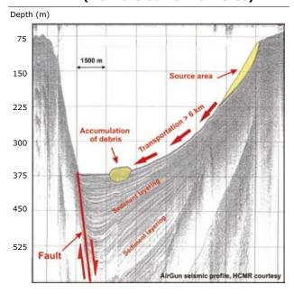
The most striking example took place on 16 October 1979 in the western Mediterranean. A large slide involving at least 8 million m<sup>3</sup> occurred in shallow water during infilling operations related to the enlargement of Nice airport at the Var River mouth. Fine to medium sand from the coastal zone was transported up to more than 200 km from the fault site (Migeon *et al*, 2004). The tsunami, which followed the collapse, drowned the coastal zone of Nice and several people were killed.
