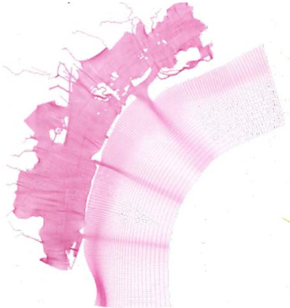
Figure 6 Example of unstructured grid for Venice Lagoon with refinement in the coastal areas and along rivers. Source: Presentation by Technital S.p.A and Deltares at the Next Generation Hydro Software Symposium, Delft, 2013.
