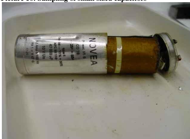
Picture 16: Sampling of small sized capacitors
