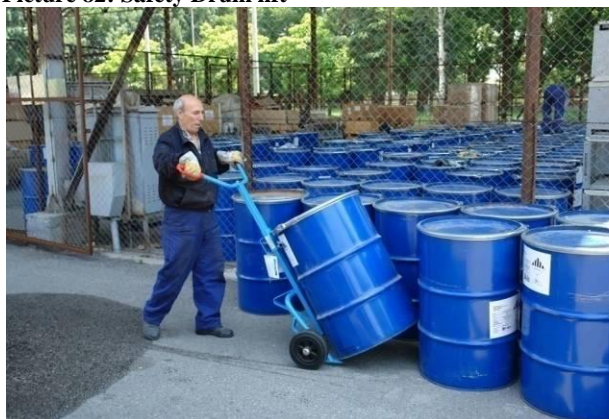
Picture 82: Safety Drum lift
