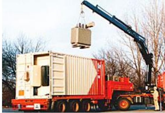
Picture 100: Loading of transformers
