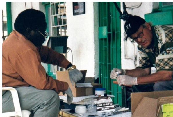
Picture 30: Use of Clor-N-Soil on Site
