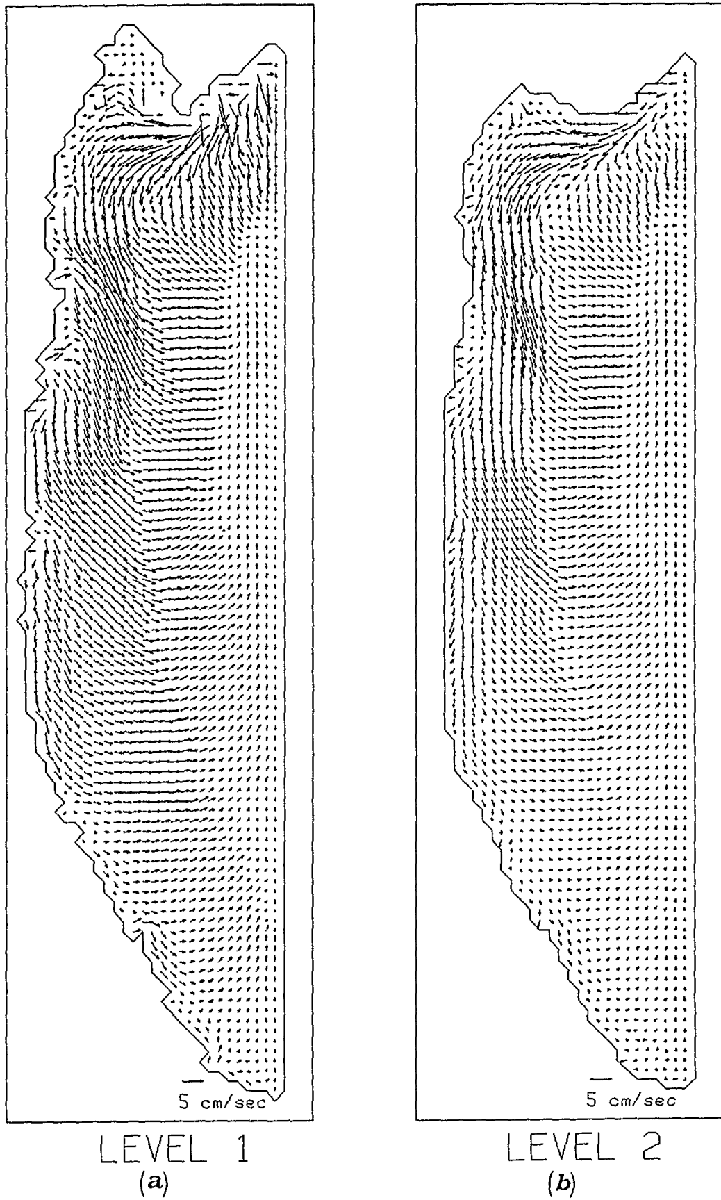
Fig. 14(a),(b). Computer simulated residual circulation patterns along Emilia-Romagna coast after 15 days. Sea current speeds are shown by the lengths and directions of arrows.
