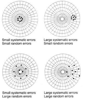
Figure 4.1: Different types of error in laboratory measurements
