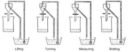
Figure 3.8: Schematic representation of an automatic free-fall sampler coupled with a fixed quantity-feeding device
