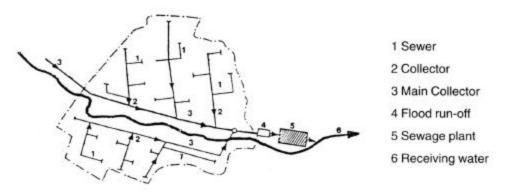
Figure 3.4: Scheme of a sewage network
