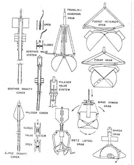
Figure 3.9: Miscellaneous bottom sediment samples.
