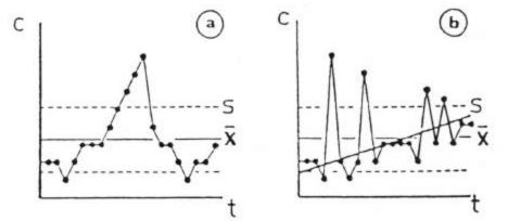
Figure 4.4: Time series of concentration of a particular chemical constituent in surface water: (a) cyclic and (b) trend.
