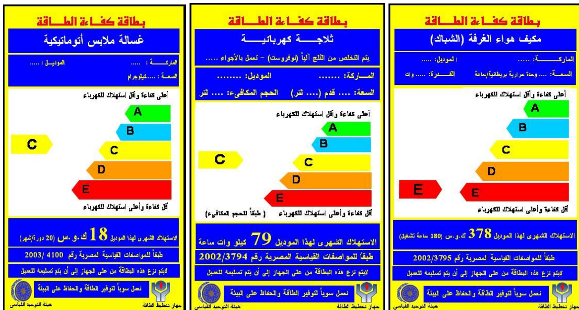
Figure 7 EEL (from the left for washing machines, window air conditioners, and refrigerators)
