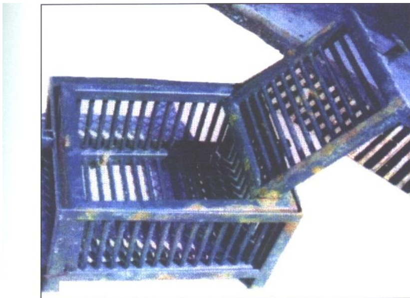
Figure 3. Cage for mussels transplantation to biomonitoring sites. Cages (marine steel, 43x48x25cm) have been built by La.Met., Lucca, Italy.
