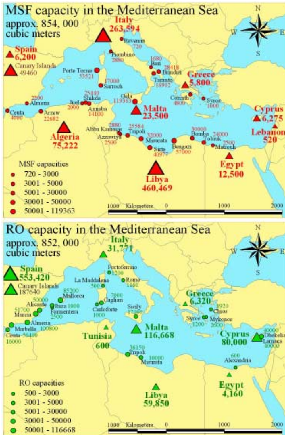
Figure 4-2: MSF and RO capacities in the Mediterranean Sea, with each process contributing about 0.85 million m 3 /day. Triangles refer to national capacities, dots illustrate capacities of selected plant locations (data based on Wangnick, 1999).
