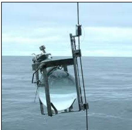
Figure 4. Glass bottle for seawater sampling for organic contaminants analysis (ICES/OSPAR 2012)
