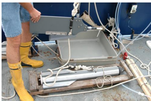
Figure 3. Surface pump sipper/tow fish system (GEOTRACES, 2017)
