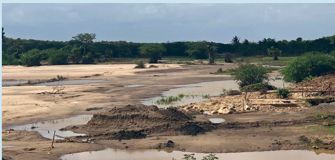
Plate 8. Sand mining as see here for the Sabaki (Athi River) Estuary can significantly affect sediment supply.
