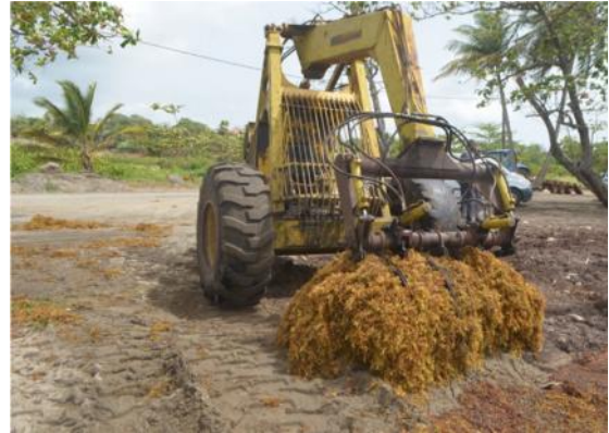
Using a cane-loader to collect large quantities of Sargassum in Guadeloupe.
