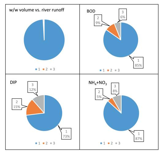
**Figure 52**. The quota of the river runoff (1), wastewaters from Primorye (2) and wastewaters from the south part of Sakhalin Is. (2) in the input to the NOWPAP sea area in terms of water volume, and contaminants: organic matter (BOD), phosphates (DIP), and dissolved nitrogen  $(NH_4+NO_3)$
