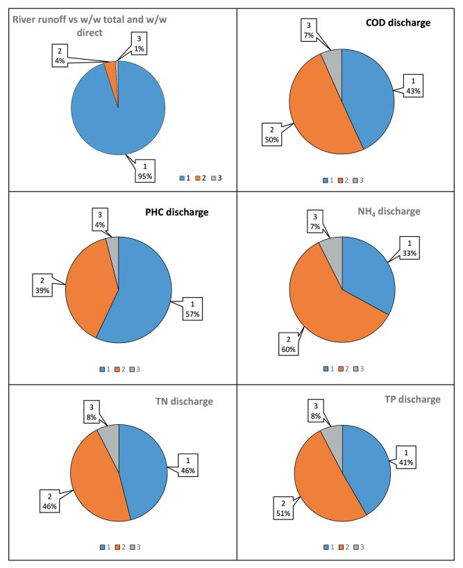
**Figure 45**. The quota of river runoff (1), wastewaters discharge (2), and direct inputs (3) from Liaoning province in terms of water volume, and contaminants emission: organic matter (COD), petroleum hydrocarbons (PHC), ammonia nitrogen ( $NH_a$ ), total nitrogen (TN) and total phosphorus (TP). (Source: China Statistical Yearbooks)
