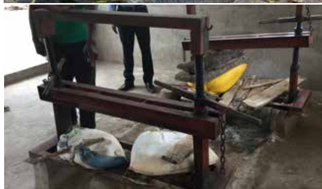
TOP: Traditional way in which women conduct pressing to extract water in the processing of gari BOTTOM: Improved method of pressing to extract water in the processing of gari in a neighbouring village Photo | SWITCH Africa Green
