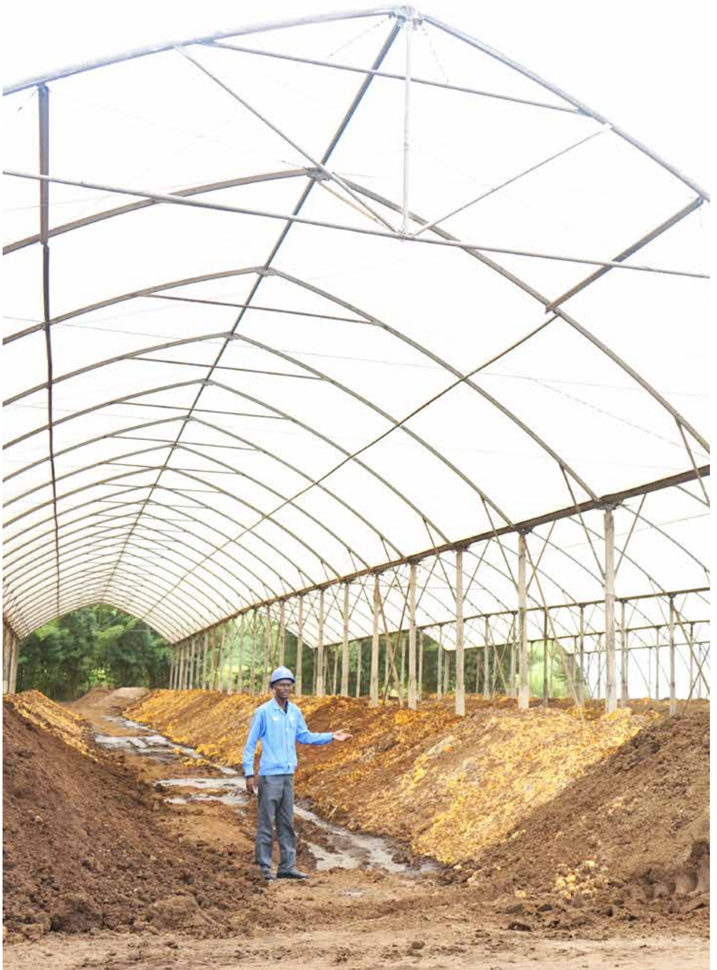
James Kunya, an employee at Sugar Company of Uganda Ltd (SCOUL) explains the process of manufacturing organic fertilizer from filter case and spent wash, raw materials from the factory that were previously disposed as waste.
