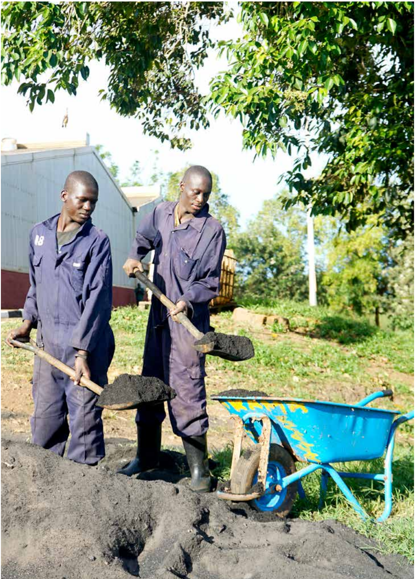
Employees at All Green Agro located in Jinja, mixing charcoal char (from a paper factory) with leather fleshings (from a tannery) to manufacture organic fertilizer. These raw materials were previously disposed off as waste.
