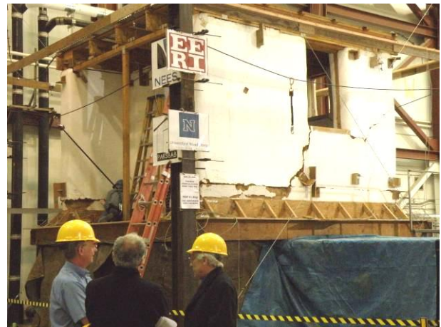
Straw-bale house earthquake simulation at the University of Nevada, Reno, US
