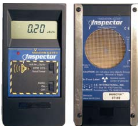
Above: Inspector Geiger-Müller instrument
