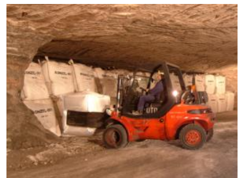
Fig. 11:Placing waste packages in an underground waste disposal facility
