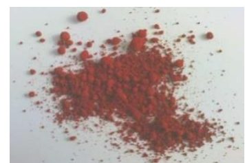
Fig. 7 Stabilized elemental mercury: red mercury sulphide (cinnabar)
