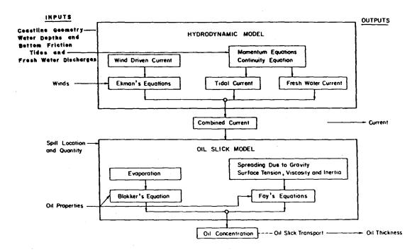
Fig. 5. General formulation of the mathematical model of an oil slick
