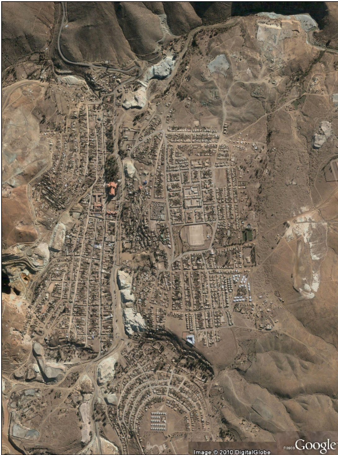
Fig. 6: Satellite image of Andacollo town. Numerous abandoned flotation ponds and tailing dumps from small scale mining (pale colours) stretch along the principal drainages (N-S: Qda. Culebrón; E-W: Quebrada Los Negritos) and dot the town ( GOOGLE EARTH 2010 ).
