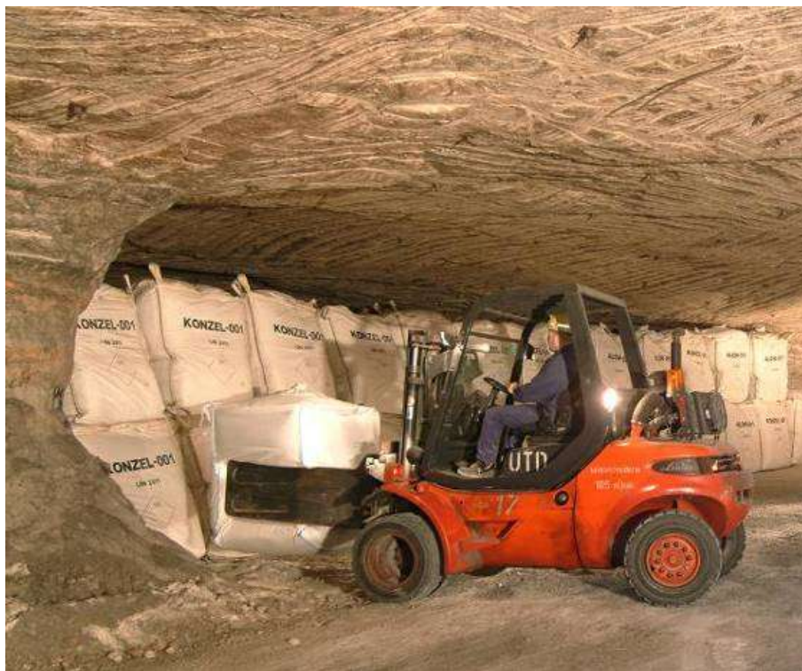
Figure 46 UTD Herfa-Neurode, big-bag disposal operation in an underground chamber (source: K+S Entsorgung [4])
