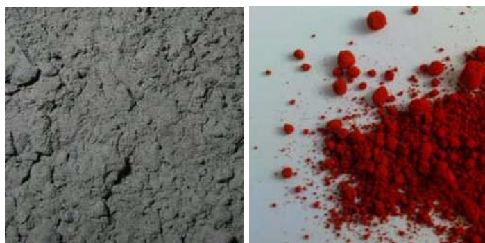
Figure 2 Black mercury sulphide (metacinnabar) and red mercury sulphide (cinnabar)
