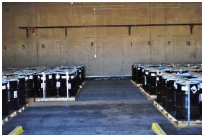
Figure 11 Storage of elemental mercury in Hawthorne (source: Rebecca Montgomery, Joint Munitions Command)
