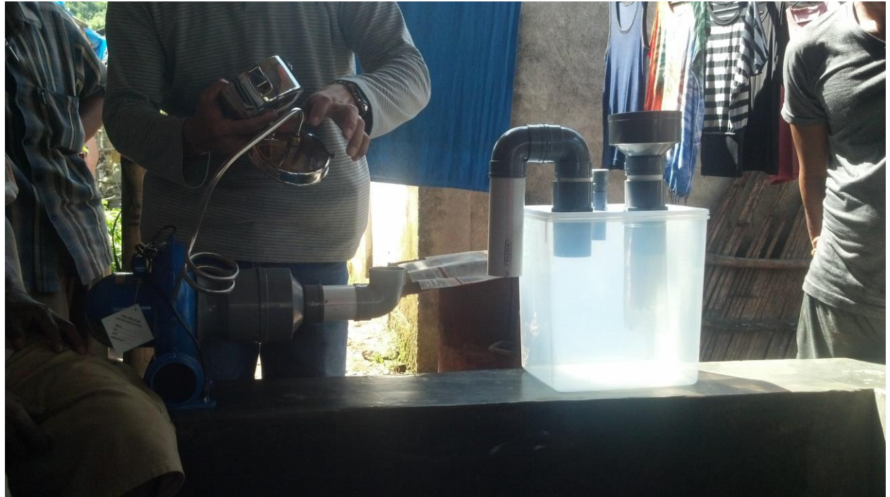
A trainer demonstrates a retort and water-box condenser to a group of local miners. These technologies can be made locally and are inexpensive to purchase. The miners were extremely receptive to using these technologies.
