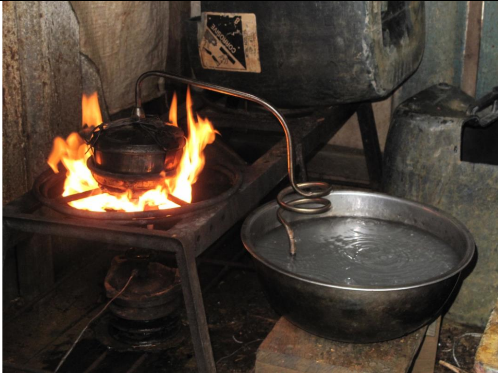
A small-retort designed and marketed by the local entrepreneur Pak Fauzi is effective for amalgam burning up to 1 kg.
