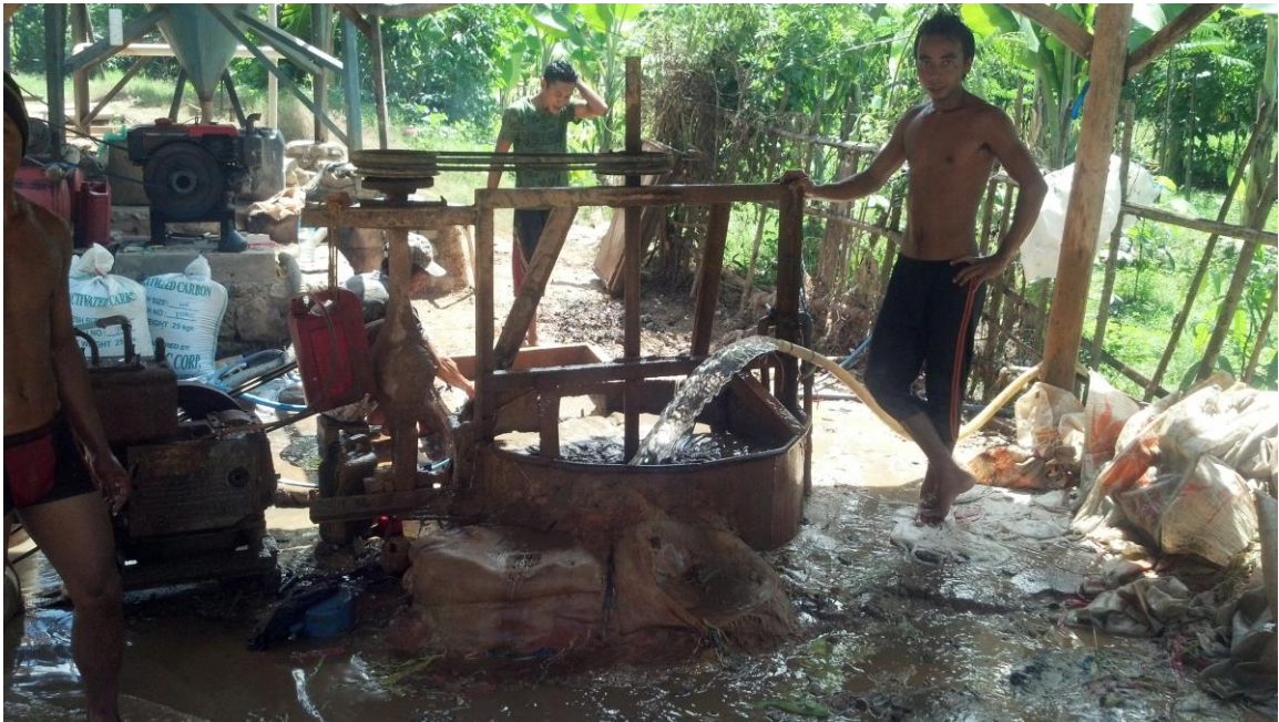
Tailings being processed by cyanidation in Lombok.
