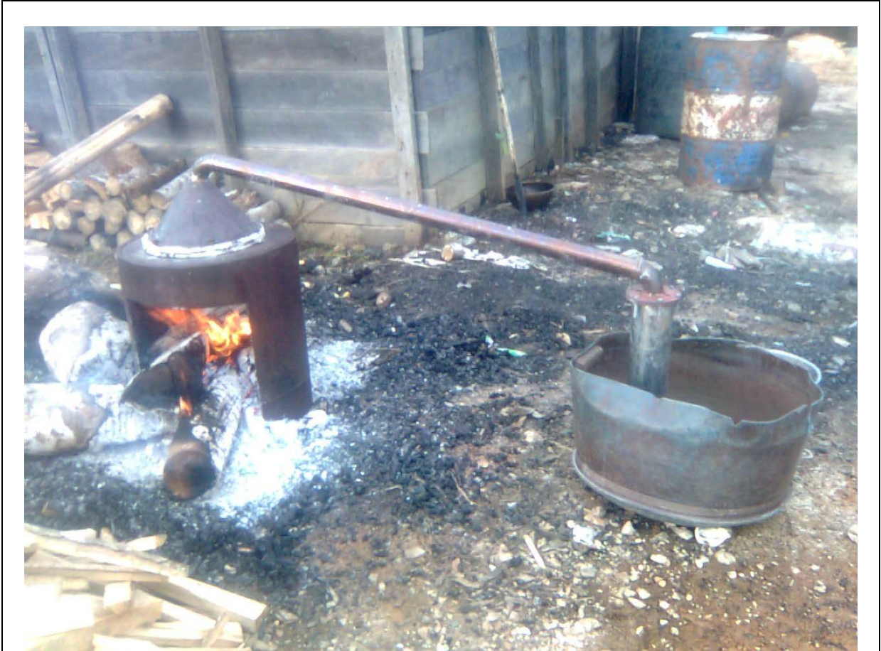
A modified large-capacity retort that is shorter than the original design, so it will fit into the stove and quicken the “cooking” time.
