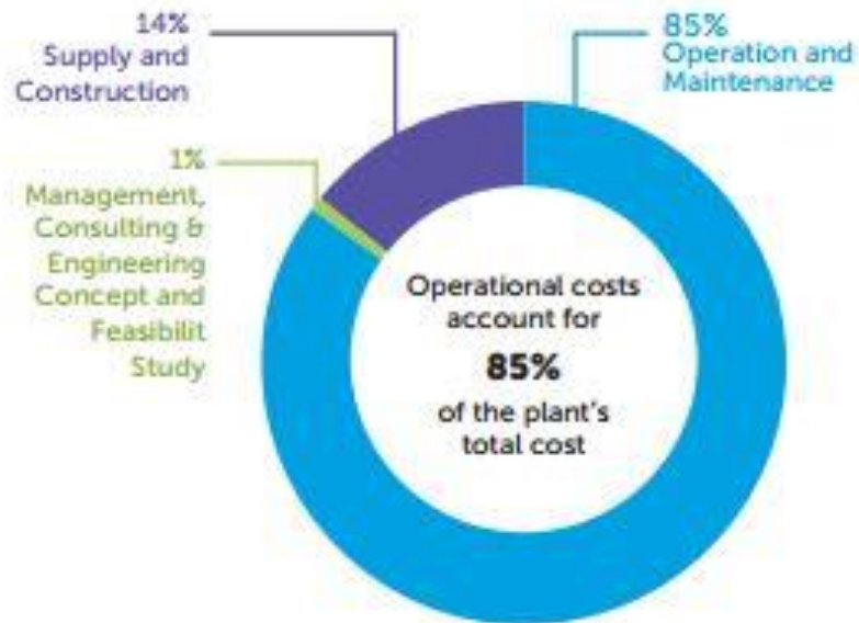
Figure 2.6 Estimated total cost of a thermal WtE plant in Europe (Neubacher 2010)
