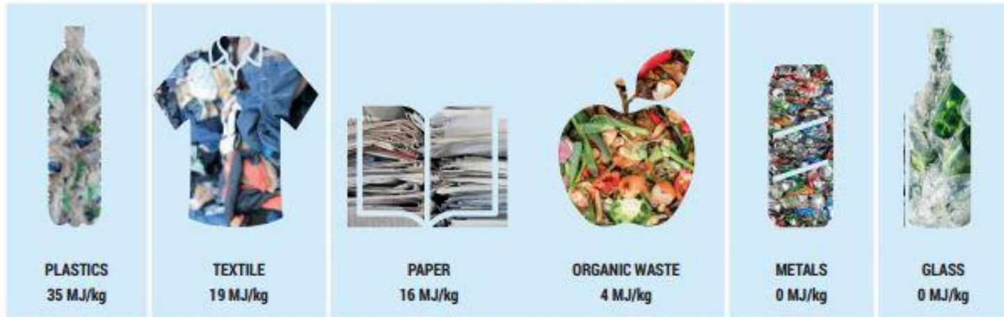
Figure 2.1 Net calorific value of different waste types found in MSW (World Energy Council 2016a)
