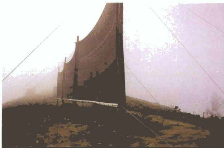
Fog-trapping nets capture moisture from the air
