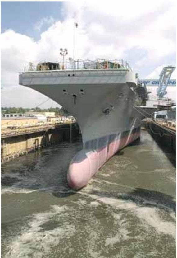
Bulbous bows provide fuel savings from reduced water resistance in naval ships.
