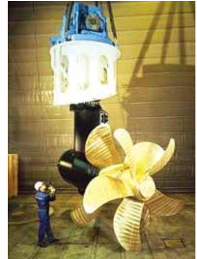
The Rolls-Royce azimuth thruster, type Contaz. In naval applications, contra-rotating propellers can improve propulsion efficiency by 5-10 percent. Rolls-Royce
