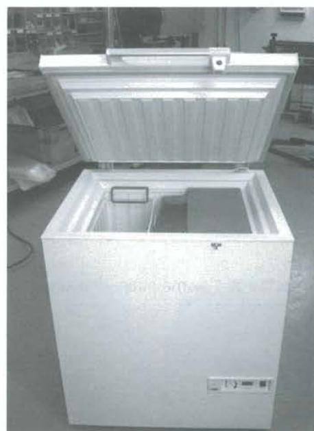
Photo1: Prototype of vaccine cooler. The vaccine will be placed in three baskets, placed vertical in the left side of the cabinet. The ice storage is placed under the blue lid in the right side of the photo. The compressor is placed in a room under the ice storage.
