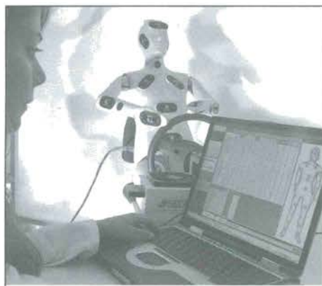
Thermal Manikin used to measure the Operative Temperature and the thermal comfort level. The manikin is produced under CRF licence by SixTau.
