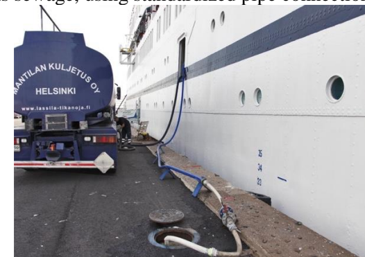
Sewage collection in port of Helsinki (Finland) (Photo credits: Clean Baltic Sea Shipping)
