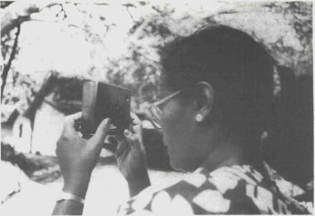
Testing for nitrate in water using a colour-match comparator
