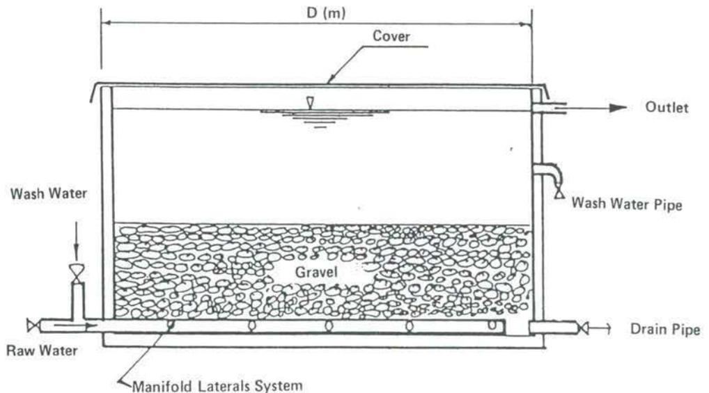
Fig. 3 Important components of upflow gravel prefilter
