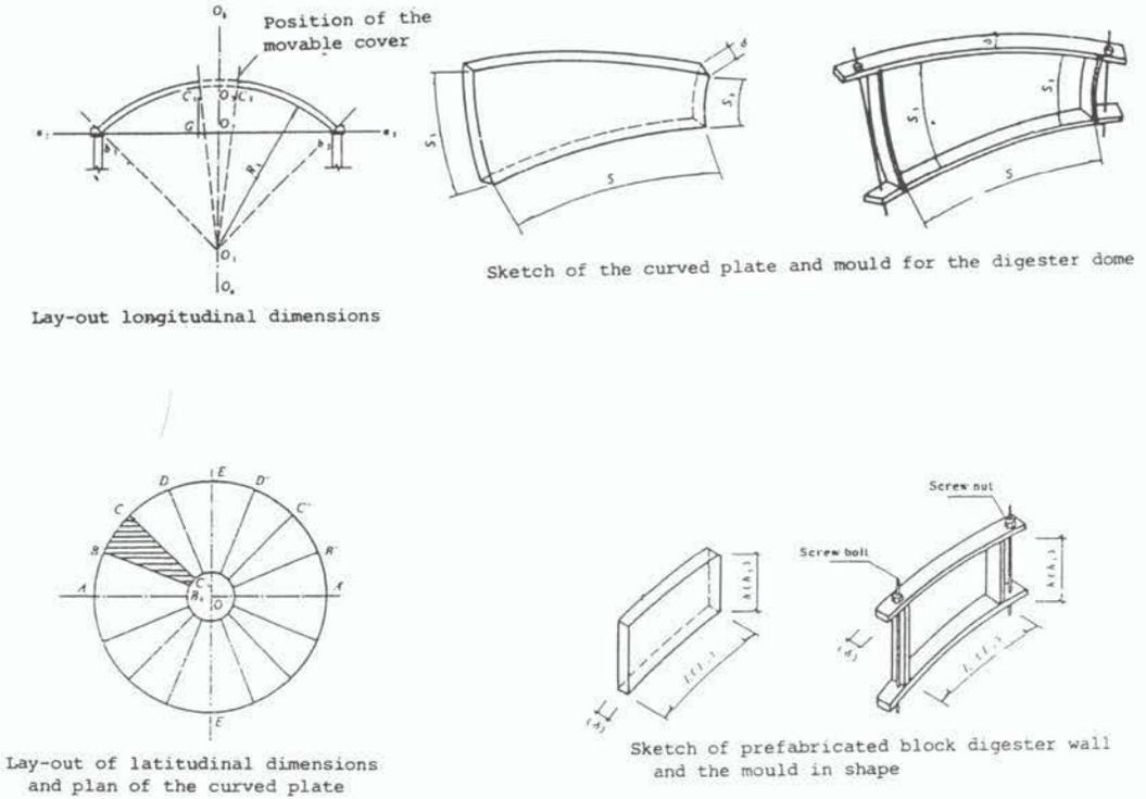
Figure 6: Molds for digester wall and dome, layout of latitudinal dimensions (14).
