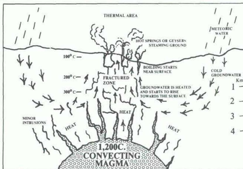
Figure 1. Model of a geothermal system showing the convection mechanism by which rising hot water is replenished by precipitation (the cycle can span hundreds of years).
