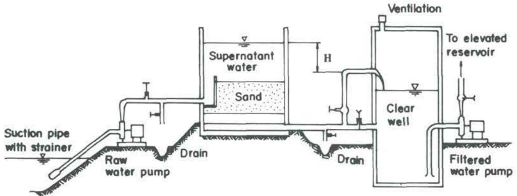
Figure 1. Simplified operation of slow sand filter
