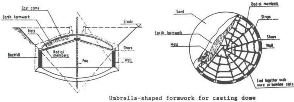
Figure 4: Construction technique for cast dome on umbrella-shaped formwork (adapted from 15).
