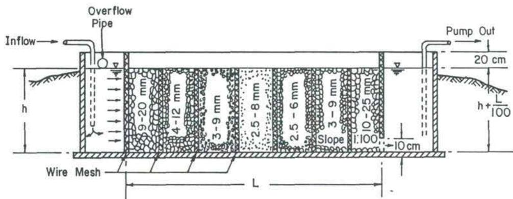
Figure 2 Horizontal-flow coarse-media filter
