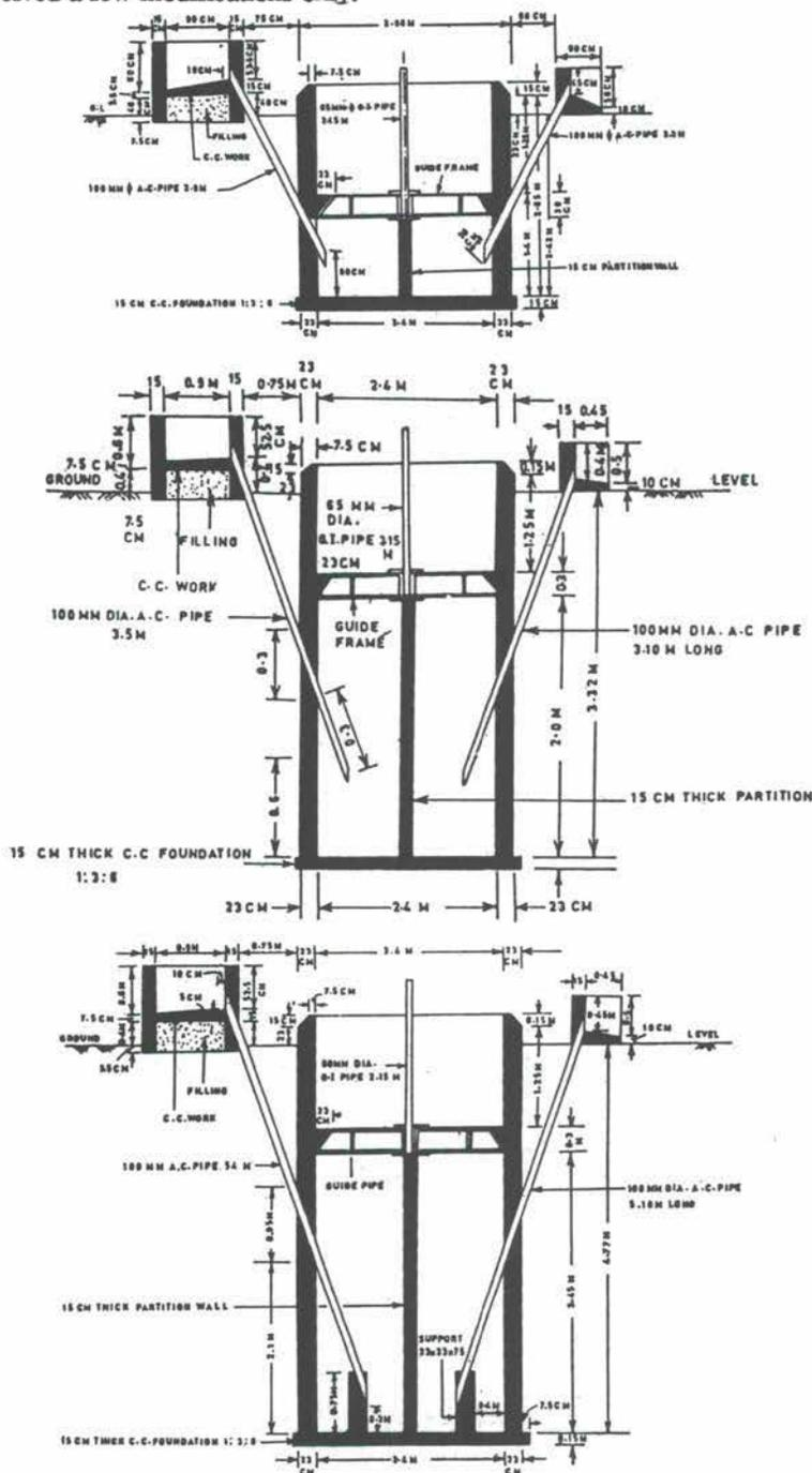
Figure 7: KVIC Plants of  $8\text{m}^3$  gas per day. Above: 30 days HRT; middle: 40 days HRT, below: 55 days HRT (adapted from 5).
