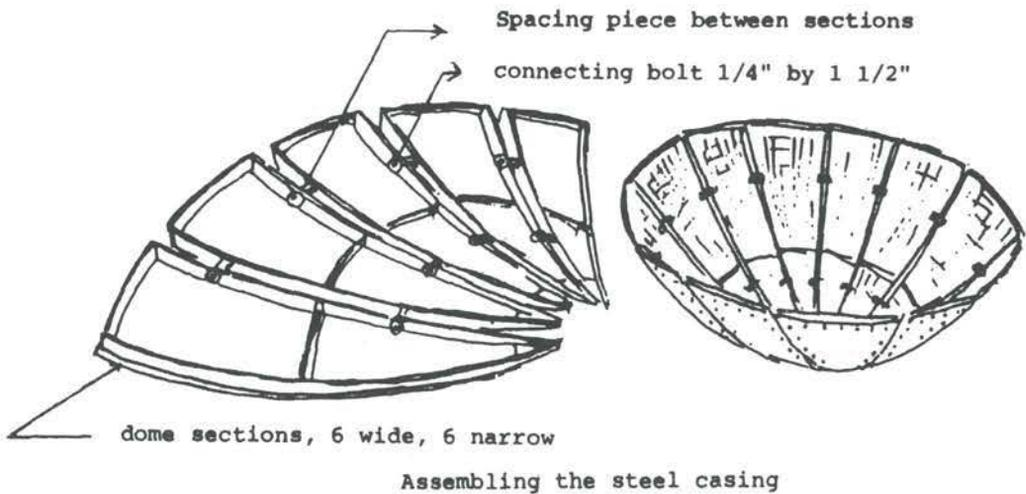
Figure 14: Assembling the steel molds for the dome (34).
