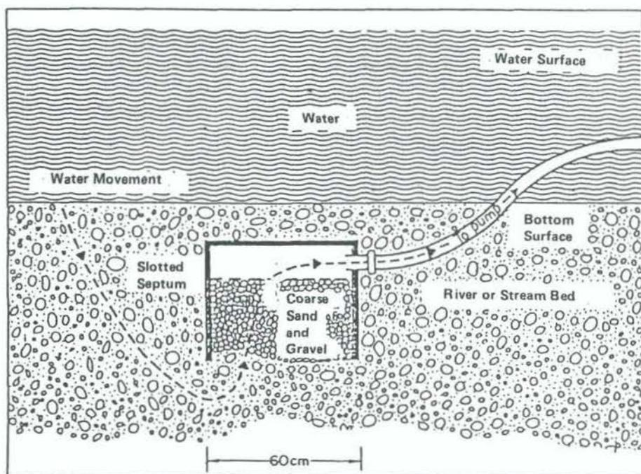
Figure 5. The SWS water filtration system
