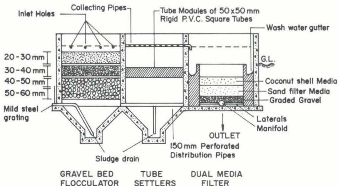
Figure 6. Flow diagram and ground-level view of upflow-downflow plant in Varangaon (Schulz & Okun, 1984)
