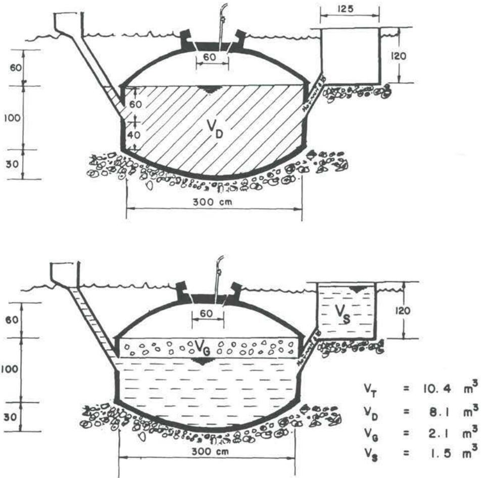
Figure 13: Fixed-dome digester designed by Department of Agricultural Extension (DOAE) (adapted from 20)
