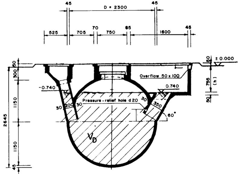
Cast-in place concrete spherical digester type I
