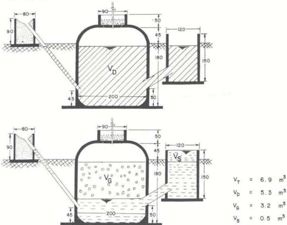
Figure 11: Fixed-dome digester designed by the Sanitation Division (adapted from 20)
