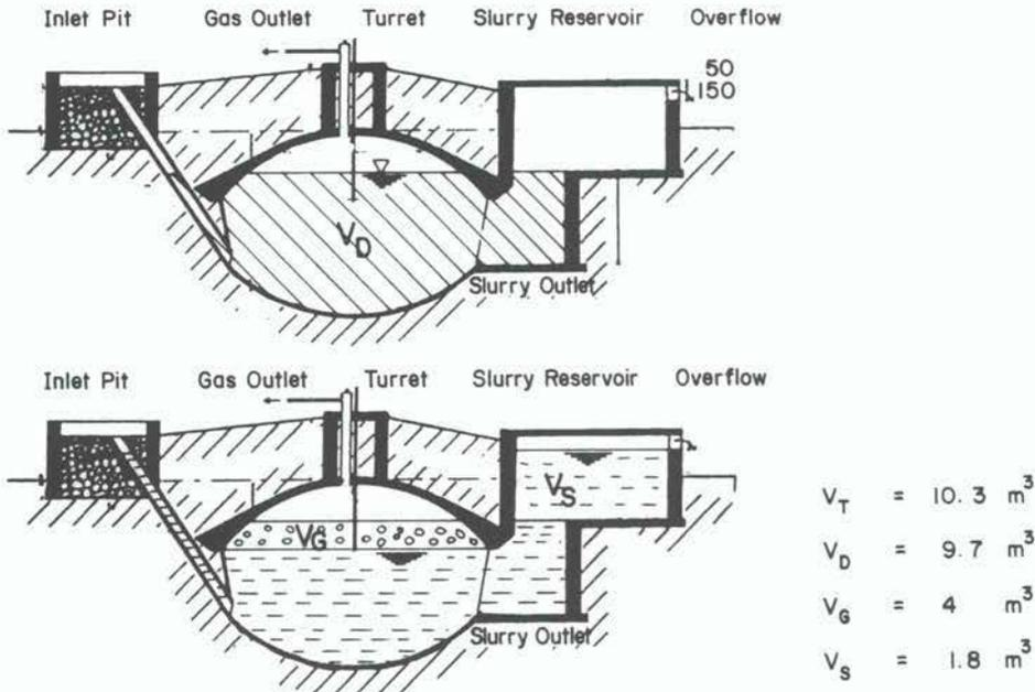
Figure 9: Design of Nepalese Fixed-dome digester, (adapted from 19)
