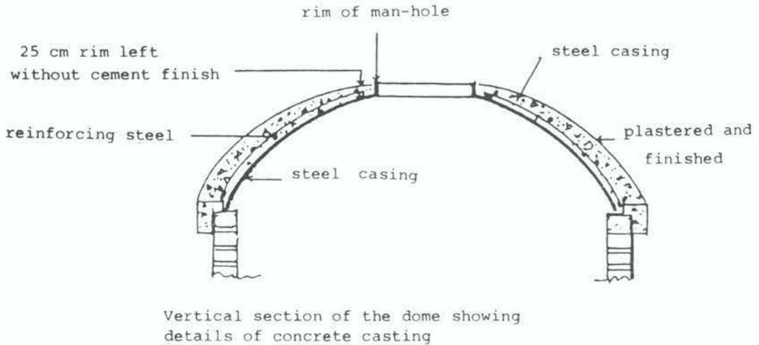
Figure 15: Finished cast-in-place dome (34)
