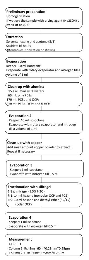
Synopsis of the analytical protocol for PCB/OCP analysis in passive air samplers
