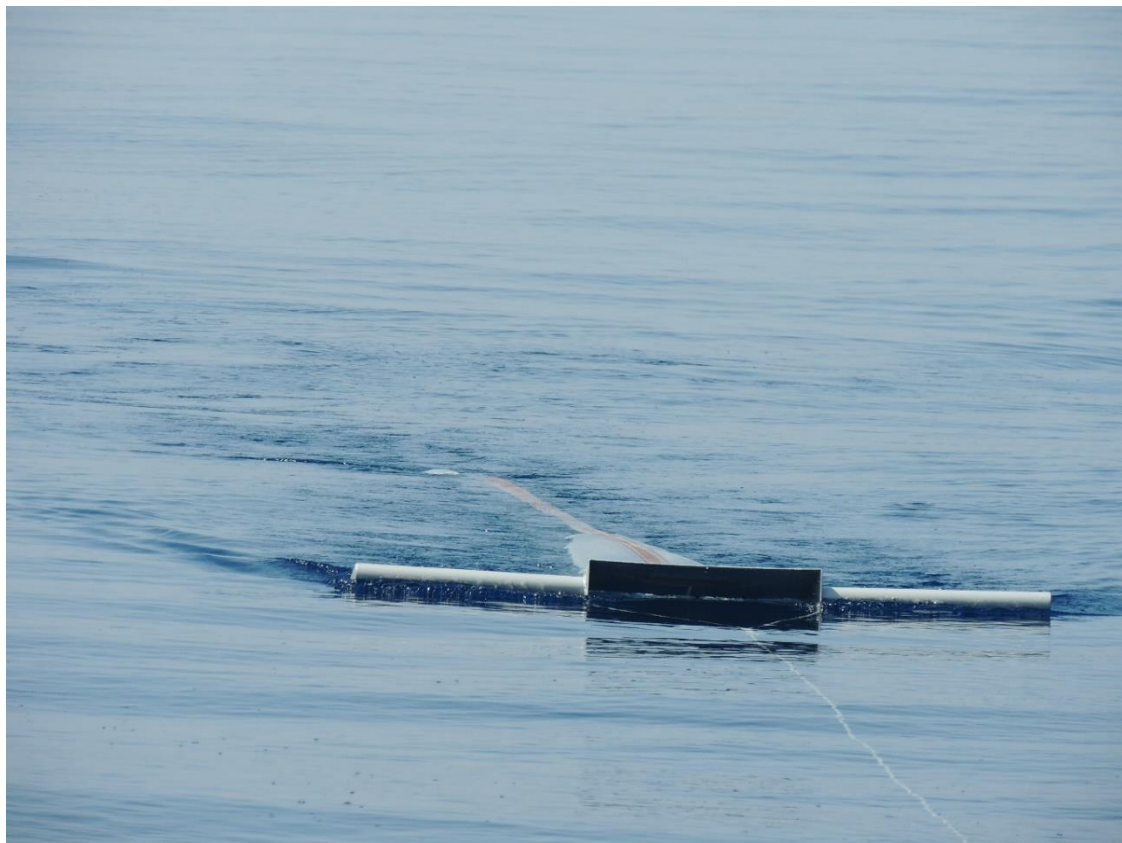
Figure 1: Manta net being operated in calm sea, outside of the bow wave caused by the spinning of the propeller (Photo: © Christos Ioakeimidis).
